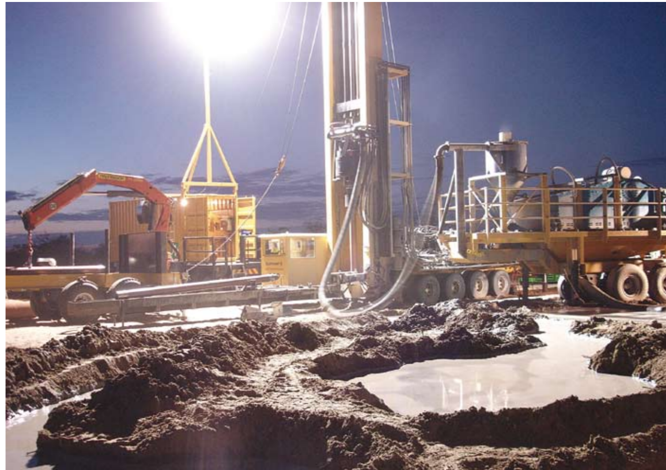
Left: Night drilling at the AK6 project using an Elephant rig. The rig drills 23 inch holes and, in effect, takes bulk samples from each hole it drills.
