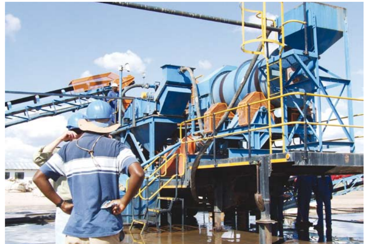
Below: This DMS plant at the exploration camp was used to process the bulk samples from AK6.
